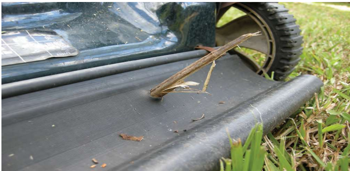
Figure 2-14. Mower guard penetrated by stick.
