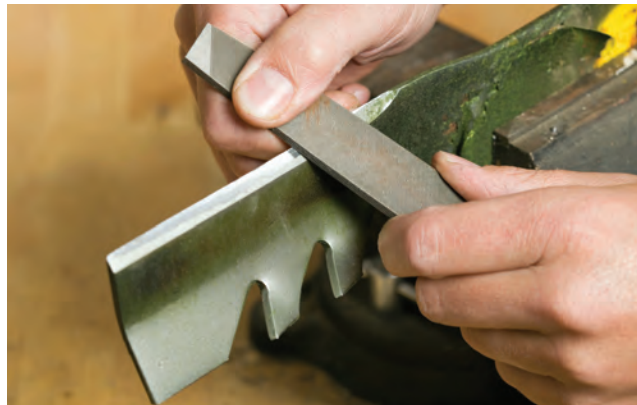
Figure 14-25. Sharpening a mower blade for a precision cut.
