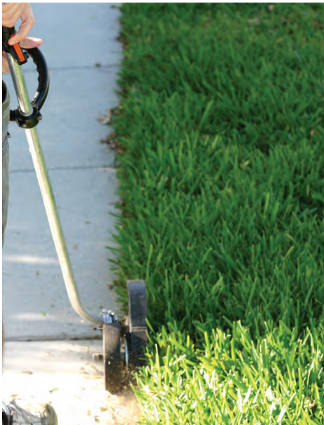
Figure 14-33. Mechanical edging to create a clean edge between turfgrass and the sidewalk.
