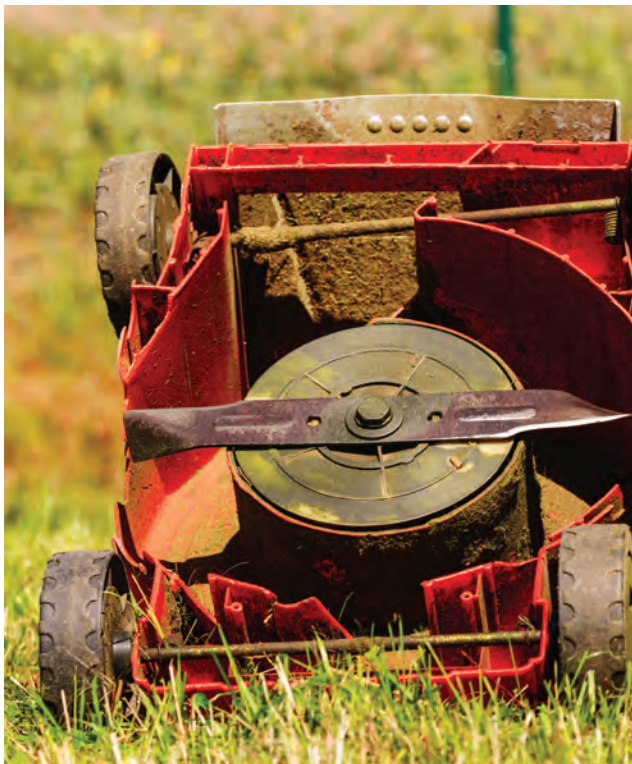
Figure 14-27. The rotating blade of a rotary mower.
