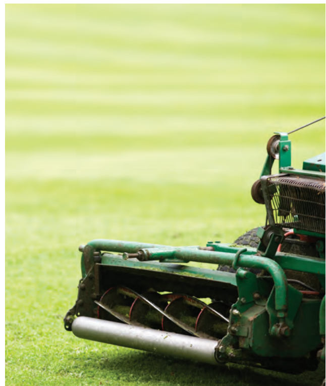
Figure 14-28. The scissor action cut of a reel mower.
