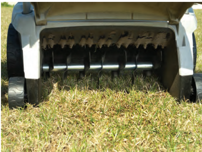
Figure 14-35. A dethatcher with vertical blades designed to cut and loosen thatch for raking and removal.
