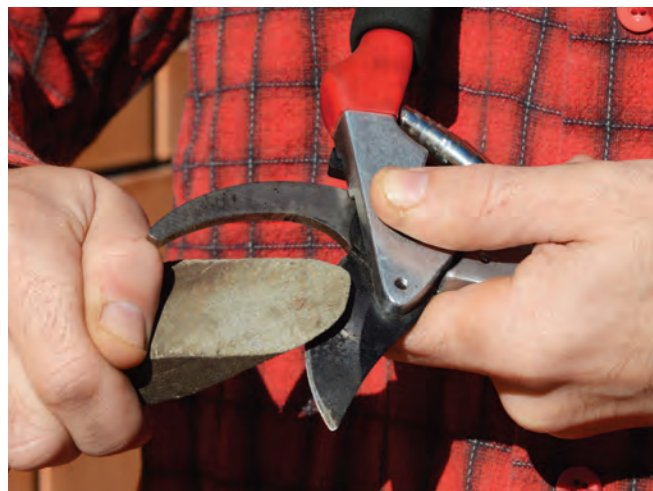
Figure 13-41. Maintaining a sharp edge on bypass pruner blades.
