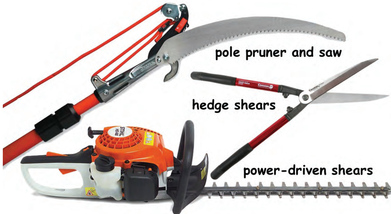
Figure 13-40. Pole pruners with saw, manual hedge shears (Corona), and power driven hedge shears (Stihl).
