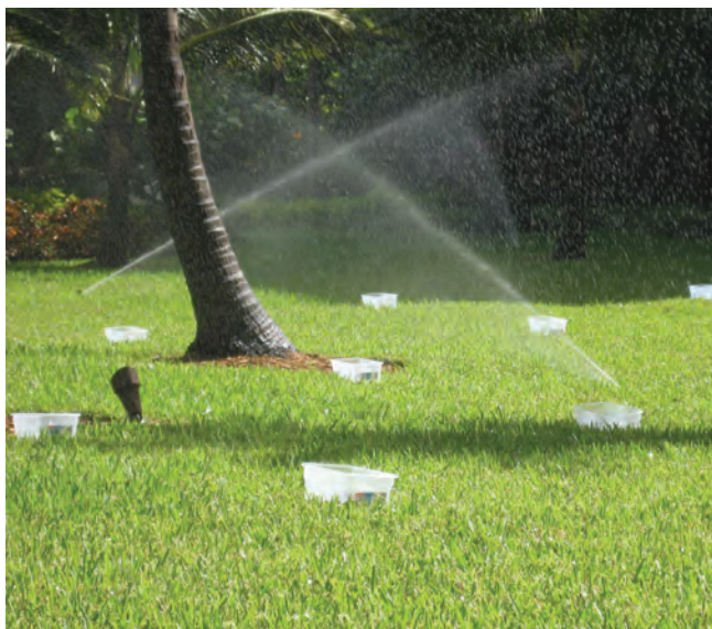
Figure 10-18. Conduction of catch can test to determine watering amount and distribution uniformity.
