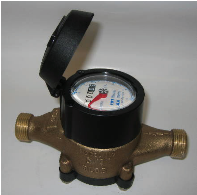
Figure 7. Inline water meter to measure water flow.
